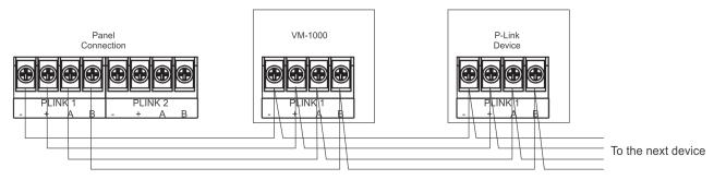
Figure 41. VM-1000 P-Link Class B Wiring Example
