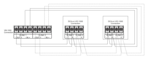
Figure 46. VM-1000 V-Link 1 and 2 Class A Wiring Example
