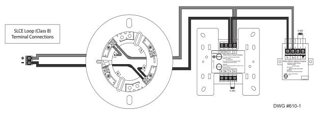
Figure 12. Nohmi Protocol Example of SLC as Class B
