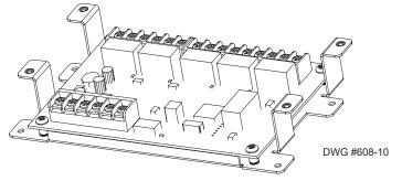
Figure 28. RLY-5 Board Showing Mounting Bracket
