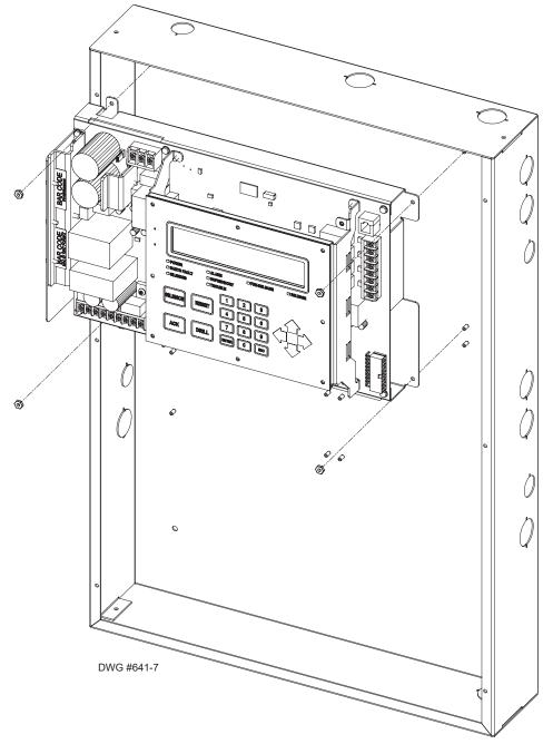
Figure 51. IPA-4000 Cabinet Showing Circuit Board Assembly
