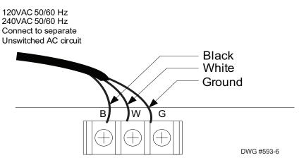
Figure 2. Main Supply Circuit
