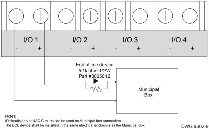
Figure 16. Municipal Box Wiring Example
