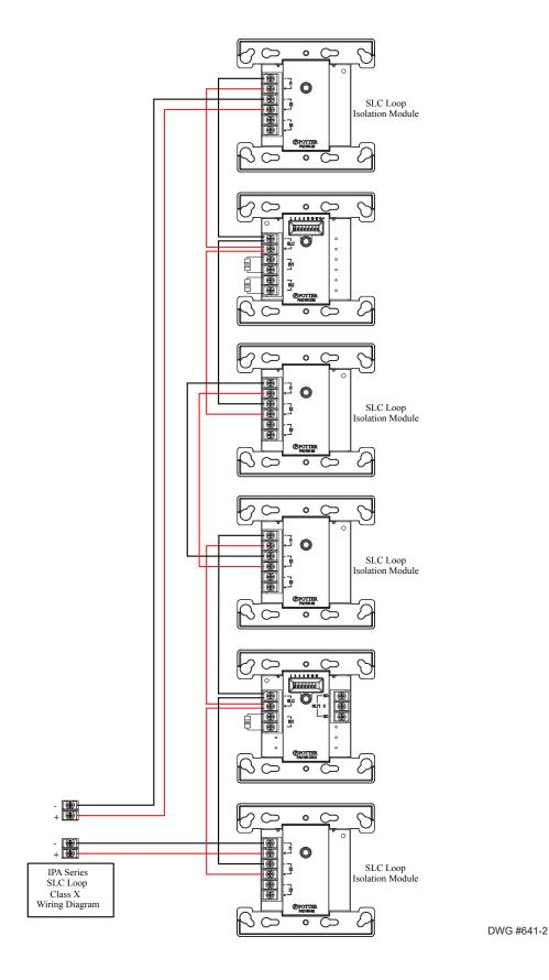
Figure 7. PAD Protocol Class X Showing PAD100-IMs Installed
