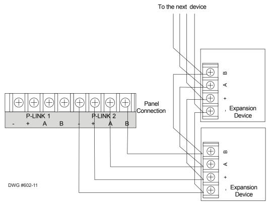
Figure 13. P-Link Class B Wiring Example
