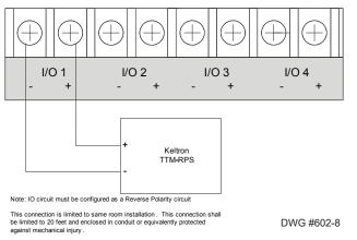
Figure 17. Example of Reverse Polarity I/O Circuit Wiring
