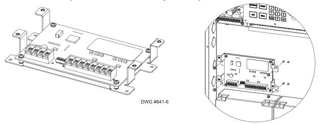
Figure 33. MC-1000 Multi-Connect Board & MC-1000 Shown Installed in IPA-4000 Cabinet
