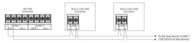
Figure 43. VM-1000 V-Link Class B Wiring Example
