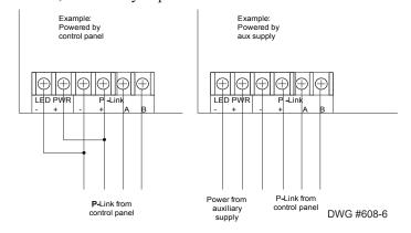
Figure 23. Examples of Wiring a LED-16/LED-16(F) Module to Control Panel or Auxiliary Power Supply
