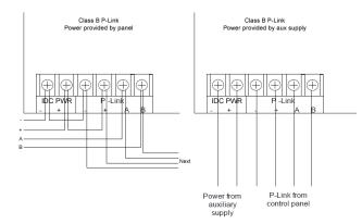
Figure 36. IDC-6 Class B Wiring
