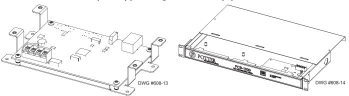
Figure 30. FCB-1000 Bridge & FCB-1000RM Showing Rack Mount
