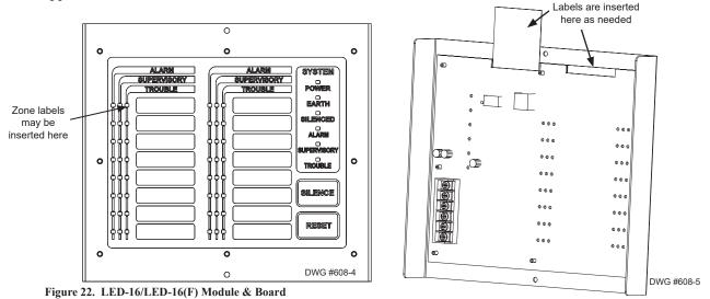
The LED-16s are controlled over the 4-wire P-Link connection. The higher current required for the LED outputs can be provided by the panel, or from an auxiliary power source as shown below. The auxiliary power can be any fire listed 24VDC source, and is fully supervised.
