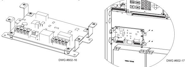
Figure 21. PAD100-SLCE / Nohmi Protocol SLCE-127 Board & Shown Installed in IPA-4000 Cabinet
