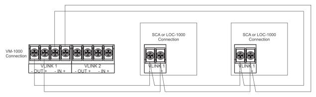
Figure 44. VM-1000 V-Link Class A Wiring Example
