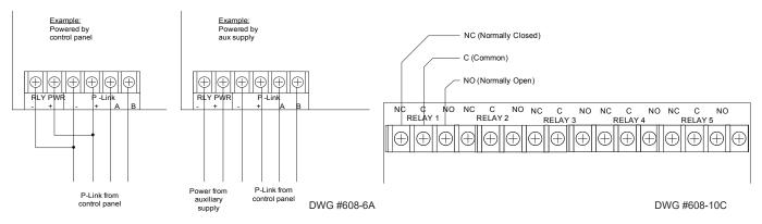
Figure 29. RLY-5 Wiring to Control Panel / Auxiliary Power Supply & RLY-5 Normally Open / Normally Closed Contacts
