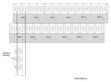
Figure 5. Class A NAC Wiring Requires CA-6500
