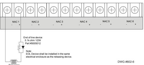
Figure Releasing Circuit Wiring with EOLD Assembly
