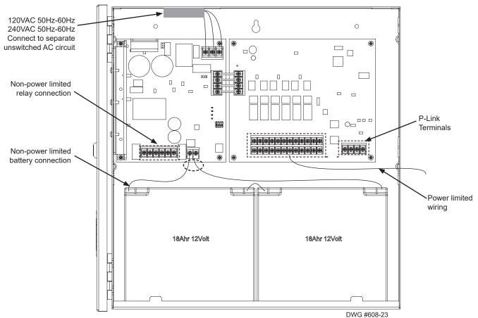
Figure 20. PSN-1000 Wiring Example
