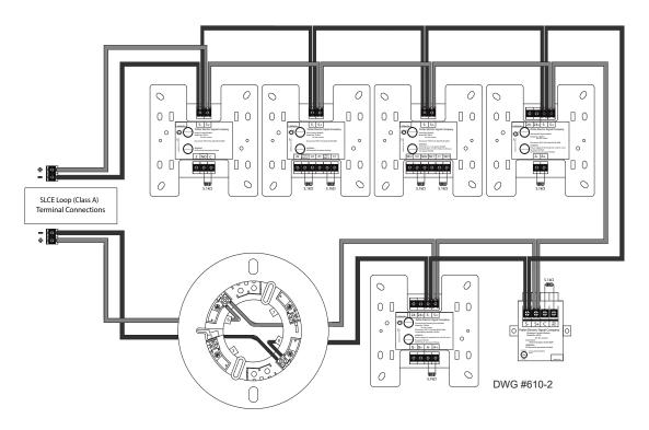
Figure 11. Nohmi Protocol Example of SLC Wired Class A
