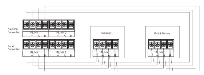
Figure 42. VM-1000 P-Link Class A Wiring Example
