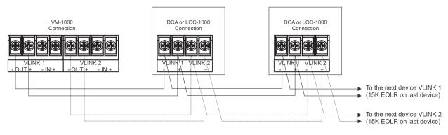
Figure 45. VM-1000 V-Link 1 and 2 Class B Wiring Example
