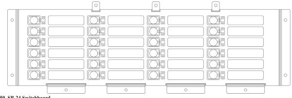
Figure 50. SB-24 Switchboard
