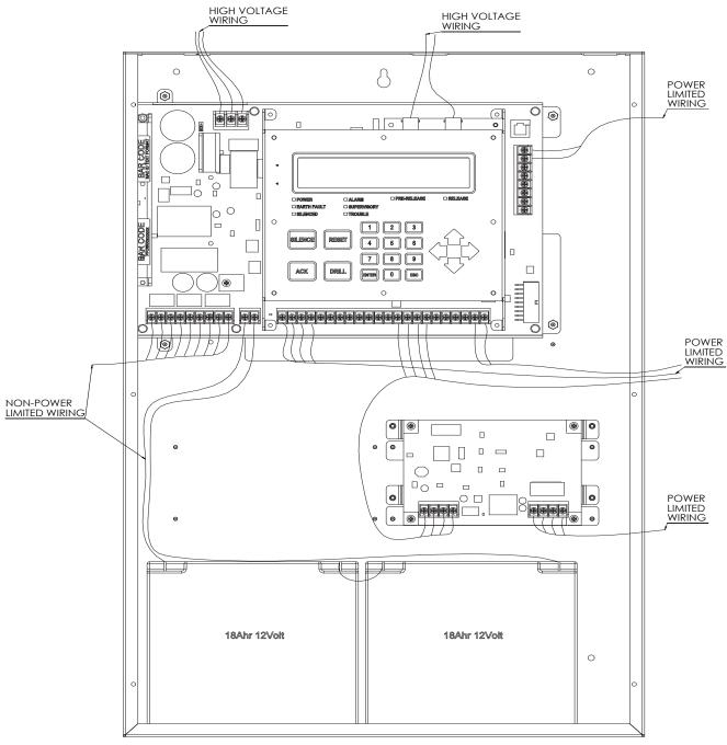
Figure 19. Example of Panel's Wire Routing
