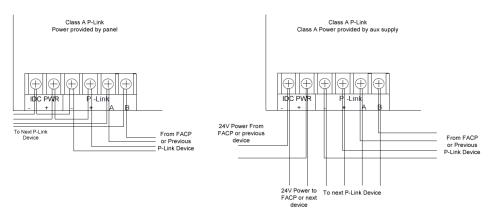
Figure 35. IDC-6 Class A Wiring
